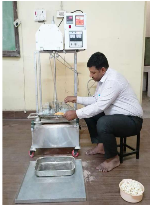
Ph.D. student working on semi-automatic multigrain popping cum puffing unit
