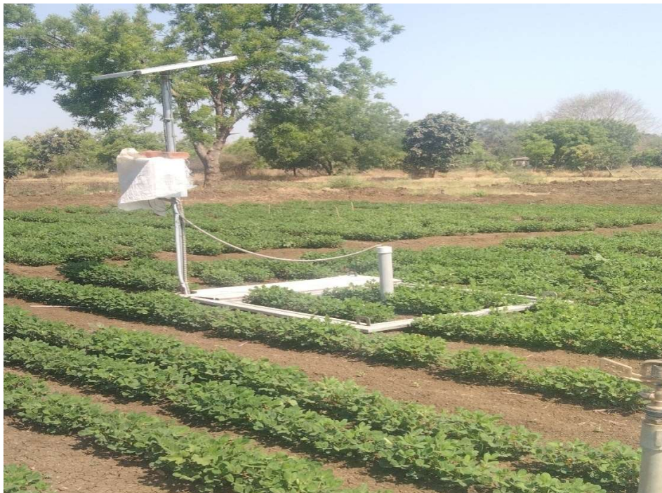
Lysimeter installed in cropped field
