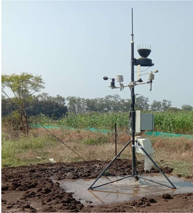
Automatic Weather Station installed in the field
