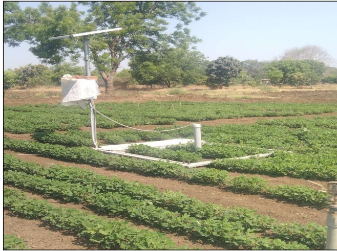
Lysimeter installed in cropped field
