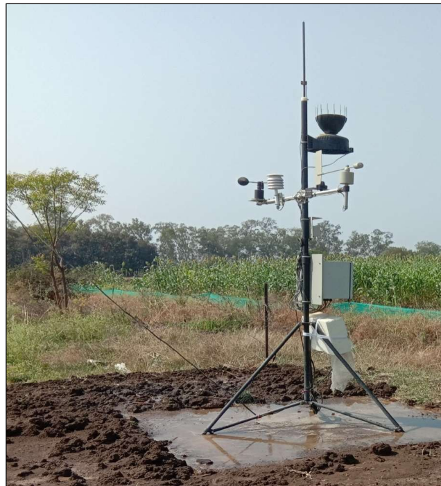
Automatic Weather Station installed in the field
